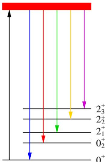
The monoenergetic beam provides separation of the ground-state transitions from the branching transitions.
