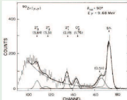
The monoenergetic beam provides separate transitions from the branching transitions.
