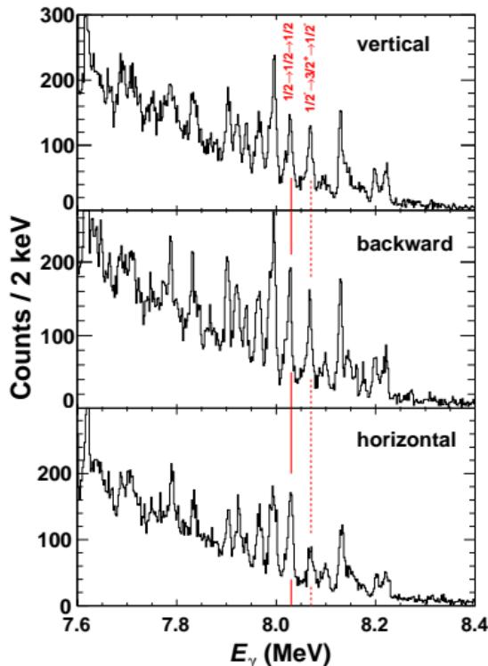
HI $\gamma$ S-Beam Properties: Linear PolarizationSpin and Parity Determination: Odd-Mass Nuclei ( $^{89}\text{Y}$ )
