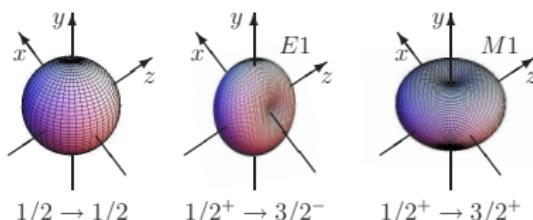
z axis: beam direction; x axis: vector of polarization
