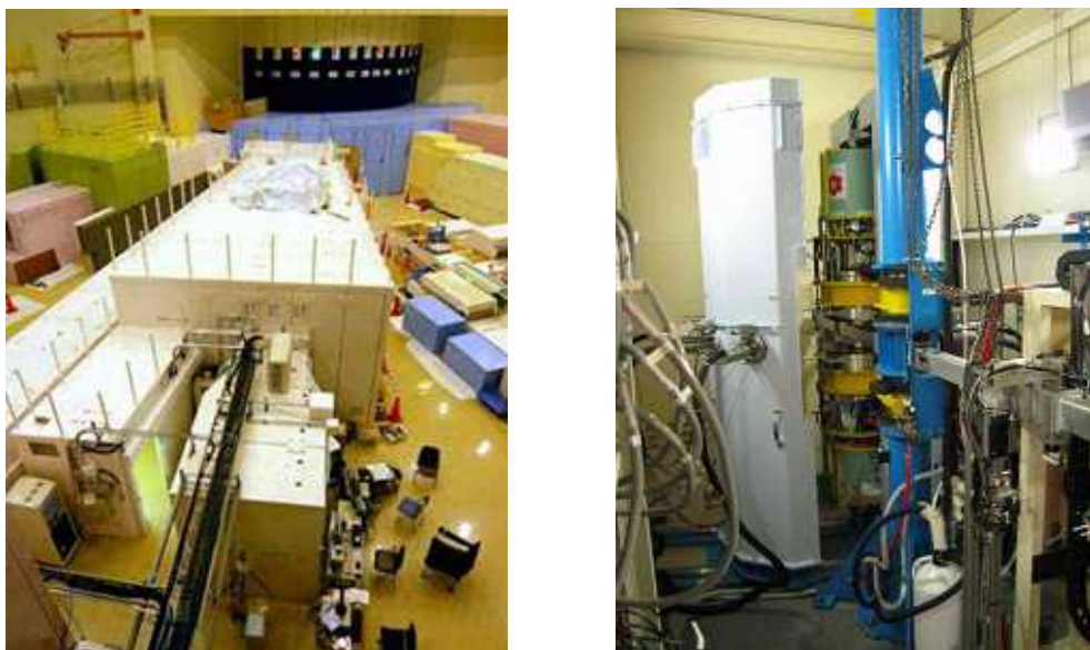
Figure 1 Photos of the ANNRI at the BL04 of the MLF in J-PARC (Left), and the "4 \pi Ge spectrometer" (Right) equipped with the ANNRI.
